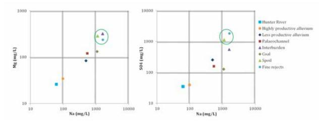
Figure 2-14 Mg/Na scatterplot and Na/SO<sub>4</sub> scatterplot of groundwater quality
