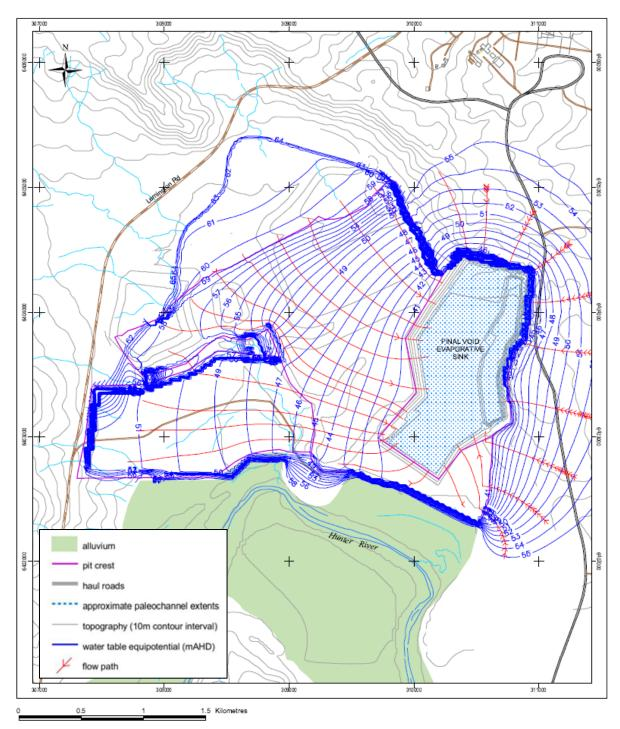
Figure 4-1 Predicted groundwater flow direction post mining (MER 2010)
