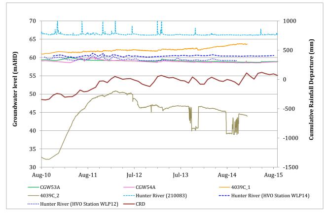
Figure 2-13 Hydrographs comparing groundwater trends in alluvium and Permian coal measures
