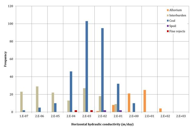
Figure 2-10 Histogram of hydraulic conductivity (Kh) distribution
